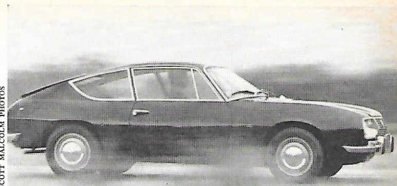
Shape of Fulvia Sport, created by Zagato, is aerodynamically excellent, improves 80-40 mph coasting time by almost 12 seconds.
